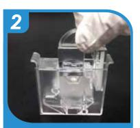
Insert reagent container into reaction cartridge.
